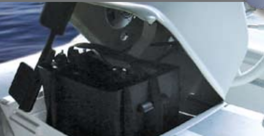
Hinged steering helm allows easy access to steering and battery compartment.
