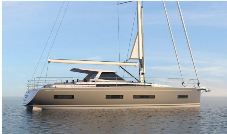
The deck line is slightly domed at the level of the main beam and has a visual effect which refines the superstructures. The front, slightly lowering part of the line increases the dynamism of the bow design. Thanks to this inverted deck line, a comfortable height can be maintained in the cockpit, in the engine room and inside the boat, such as in the galley.
